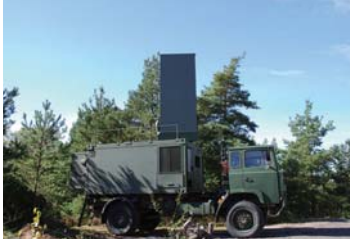
Counter-battery Detection Radar: a system that locates enemy launchers by detecting enemy shells whilst in flight.
