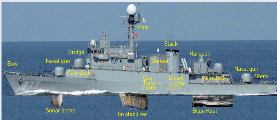
Figure 9. Overall shape and structures of ROKS Cheonan
