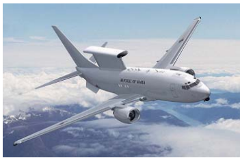
Airborne Warning and Control System (AWACS): early warning, aerial control and real time intelligence dissemination is possible across the entire Korean Peninsula.
